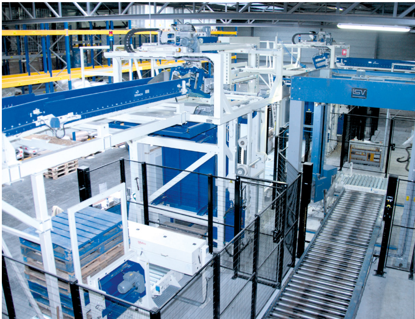
Palletizing machine with decentrally controlled asynchronous drive systems
