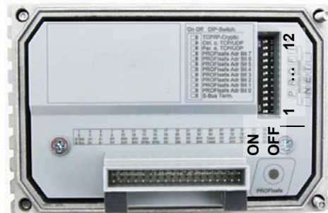
Factory settings DIP switches: OFF
