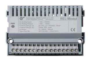
The terminal strip is divided into two potential levels (potential separation max. 50 V DC). On delivery, these are connected together with a plug-in jumper.
