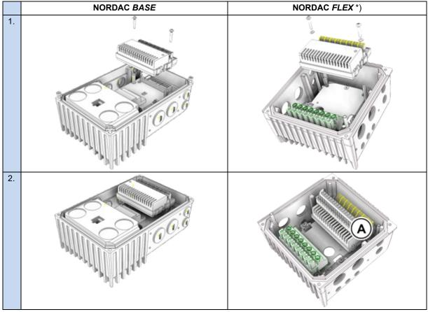
Before carrying out installation step 1 it may be necessary to remove the control terminal bar ( A ), The control terminal bar ( A ) must be fitted after installation step 2.
