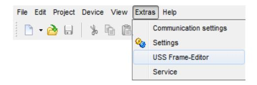
The USS Frame Editor was developed to generate and analyse USS telegrams. It is fully integrated in the NORDCON user interface and is opened via the menu item "Extras/USS Frame-Editor". The editor displays the master and slave telegram in several views. Via the tabs, the user can switch between the 9.1 "Master (order)"and the 9.2 "Device (response)".
