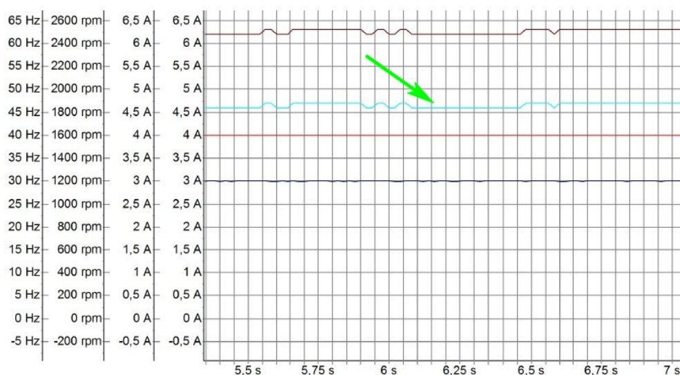
Fig. 58: Example of an optimised reluctance angle
